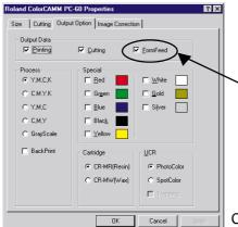
Make sure to always select [FormFeed] when printing tile page. And if there is cutting data, select [Cutting] and set the suitable [Process] depending on data.
